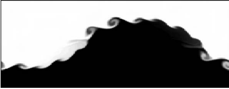
Figure 4.21. Billows growing on an interfacial wave: a numerical simulation of billows growing at the crest and trough of an internal gravity wave travelling along a density interface. (From Fringer and Street, 2003.)
