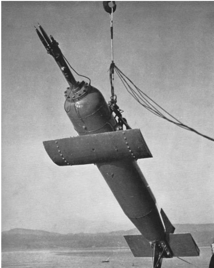
Figure 2.9. The towed paravane carrying the hot- and cold-film thermistors, visible at the top on the left, used to obtain the first records of small-scale turbulence and to determine its spectrum. (From Grant et al. , 1962.)
