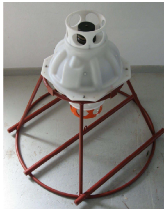
Figure 2. PACT bottom unit and steel stand. The black cylinder at the top is the HAM.NODE modem; the burn-wire release of the BU is located in the lower cage. For deployment, additional weights are attached between the release and the steel stand.
